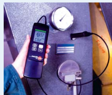
Measuring the CO 2 conc. in ingoing and outgoing air ducts
